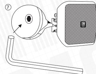
Use the hexagon key to tighten bracket angle adjusting screw.
