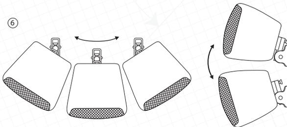
Loudspeaker's angle can be adjusted according to vertical and horizontal axis.
