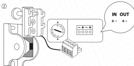
Connect the audio cable to the Euro block connector and the socket.
