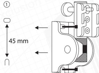
Drill the holes according to the drawing.
