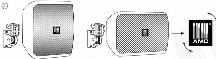
Place loudspeaker on the bracket. You can fix loudspeaker vertically or horizontally. The logo can be adjusted according to the loudspeaker's axis. To remove the bracket pull out the plunger first, then remove the loudspeaker from the bracket.
