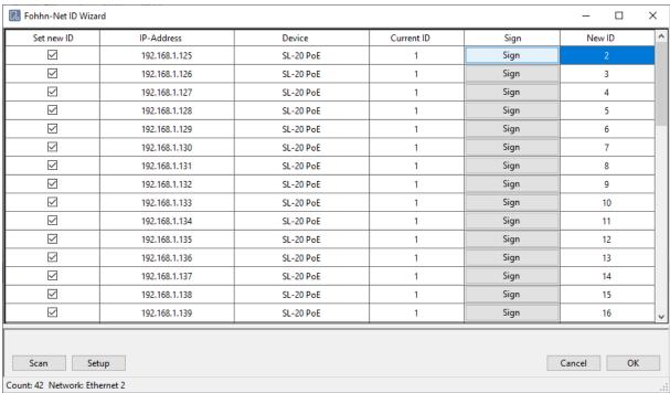
With the  ${\it Sign}$  function, you can make the blue LED in the PoE loudspeaker flash.
