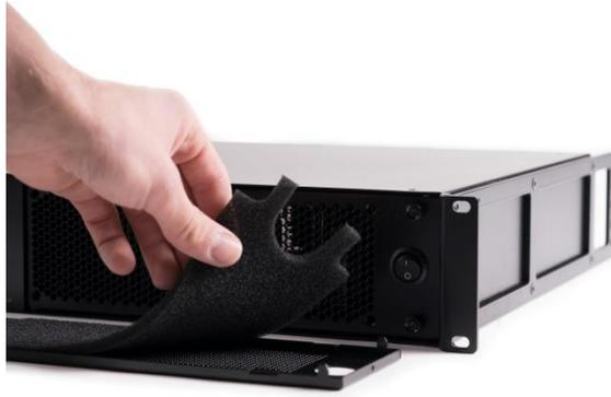
3. Put the cleaned filter foam back in the filter holder and re-attach the front panel to the front of the enclosure.
