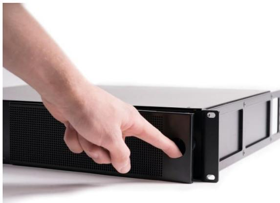
2. The filter foam that is to be cleaned can be found in the front panel's fan filter holder. Remove this filter foam and clean it, e.g. by blowing on it.
