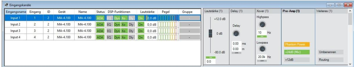
If the +24dB (Mic) switch is active, the respective input is configured as a microphone input and a microphone preamplifier is activated for the channel. The input impedance is 10kOhm. The input gain of the preamplifier is +24 dB and can be increased to +36dB with the +12dB switch. A +24V phantom power can be switched on with the phantom power switch.
