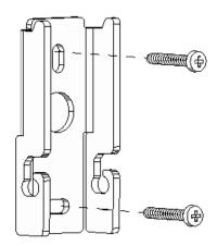
Mount the wall plate to the wall. Make sure all screws and dowels as well as the wall itself are suitable to carry the weight of the speaker. (Screw diameter max. 5 mm)
