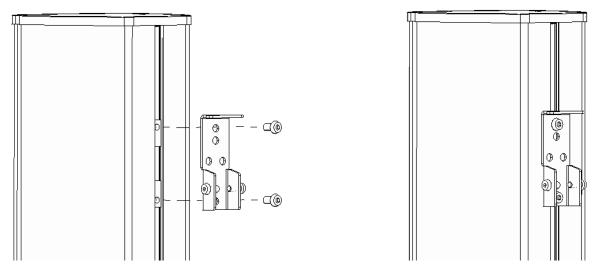
Vertical speaker position: WS-1 housing plate may be positioned anywhere at the length of the cabinet. For speakers longer than 1,3 m it is recommended to use one WS-1 on each end.
