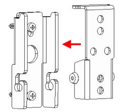
Mount the wall plate to the wall. Make sure all Insert the speaker with its housing plate into the wall screws and dowels as well as the wall itself are plate. (Picture shown without speaker.)
