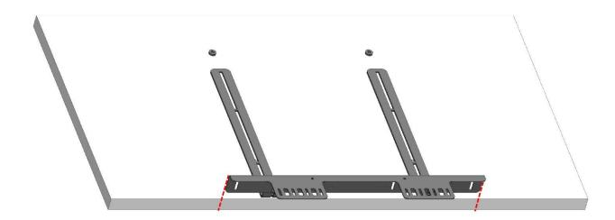
Put the VESA-Bracket-D against the rear of your display and align it with the display's outer edge as shown. For VESA threads not covered by the bracket, two 5 mm spacers are necessary.
