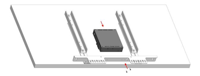
Attach a Fohhn system amplifier (e.g. MA-4.100) to the bracket.
