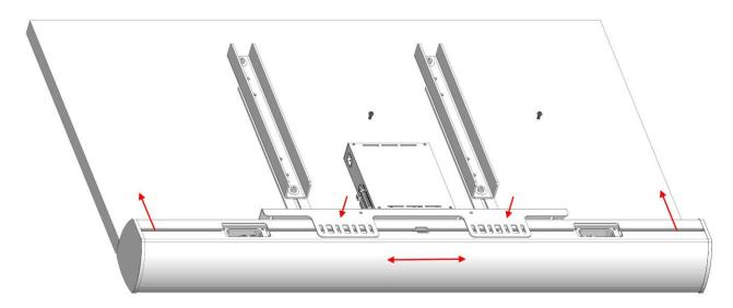
Push up the speaker against the display and align it horizontally. Bolt the speaker to the VESA-Bracket-D using the slot nuts and two M6 Allen bolts.
