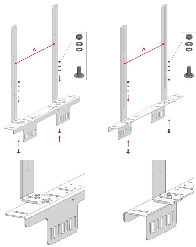
Arrange the three bracket parts according to the images in 1. or 2. If depth of display is smaller than or equal to 90 mm, refer to image 1., otherwise to image 2. Choose dimension "A" according to your display's VESA standard (200, 300, 400 or 600 mm). Screw the parts together using carriage bolt, tooth lock washer, washer and nut.
