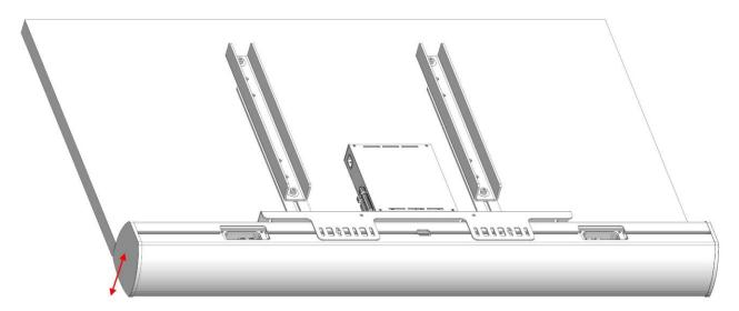
If desired, align the speaker in its depth to level with the display's screen. Please refer to 1. or 2. Make sure all screws and nuts are tightend correctly.
