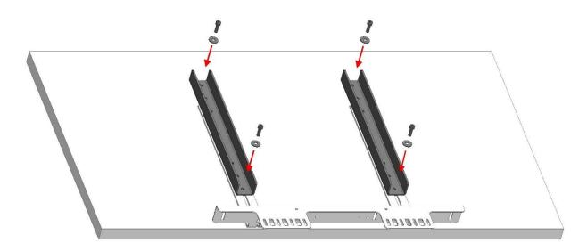
Place the VESA wall mount kit of the display on top of the VESA-Bracket-D and screw them together using Allen bolts and washers.
