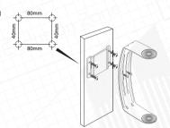
Drill holes according the drawing.
