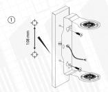
Drill holes according the drawing.
