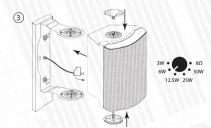
Place loudspeaker to the bracket and tighten by bracket knobs. Connect Phoenix connector to socket. Set the desired loudspeaker power tap.
