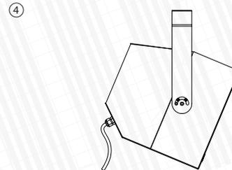
Fix the loudspeaker to the wall. Set required angle and tightened screws on the bracket.
