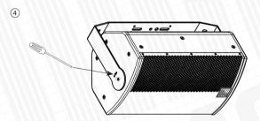
Fix loudspeaker angle with self-driving screws on both sides of the bracket. It is necessary to use these screws to keep loudspeaker from shifting angle due to weight and vibration.
