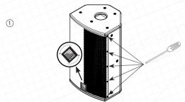
When mounting RF 10 horizontally, AMC logo and horn (tweeter) can be rotated sideways. Unscrew loudspeaker grill and loosen the screw holding the logo plate. Unscrew the horn to rotate it.
