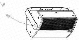
Place loudspeaker into the bracket and tighten the screws on both sides. Plug audio cables and make final angle loudspeaker adjustments.
