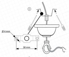
Route the cable through all parts of mounting bracket.
