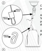
Connect provided steel rope to the mounting bracket and the speaker.
