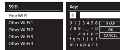
Backspace, OK, and Cancel are located to the right of the password screen. These menu options can be achieved using the rotary encoder or pressing the MENU/INFO button. The MENU/INFO button allows an instant jump to the Backspace option and back again.
