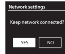
**Keep network connected:** This option keeps the network connected even if the Live radio stays in standby mode.
