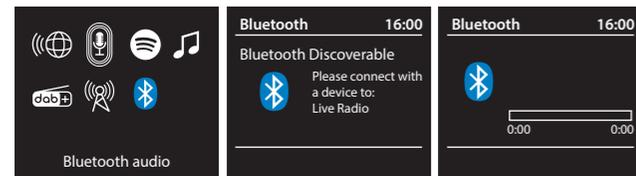
**Pairing Bluetooth:** The flashing Bluetooth icon indicates that receiver not paired to the Bluetooth device. To pair, select the option to add a new Bluetooth device on your smartphone according to your smart device instructions. Live radio will be displayed on the list of available devices that appear on the mobile device screen. Your mobile device will connect automatically once pair. After pairing Bluetooth icon stops blinking.
