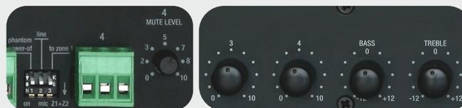
Input 4 is Zone 1 microphone input which can be assigned to both zones. It features voice over priority. With „4 mute level“ knob on the rear panel you can adjust Input 4 threshold. It also features +24V Phantom Power and can be switched to support Line level signal. Tone can be adjusted via combined Input 3 and Input 4 tone controls.
