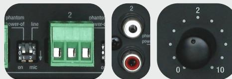
Input 2 is assignable Zone 1 and Zone 2 input. It is intended to be used with Line level signal devices, but it has ability to accept signal from dynamic or condenser microphones. Stereo RCA connector is disabled when input is configured to microphone level signal. Input level is adjusted via front panel knob „2“.
