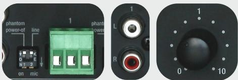
Input 1 is assignable Zone 1 and Zone 2 input. It is intended to be used with Line level signal devices, but it has ability to accept signal from dynamic or condenser microphones. Stereo RCA connector is disabled when input is configured to microphone level signal. Input level is adjusted via front panel knob „1“.
