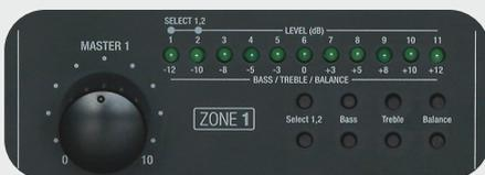
iMIX2 offers separate bass, treble, balance and master volume controls for each zone. Adjusted item values are being displayed in an indicator bar. Initially indicator bar displays zone master volume. „Select 1,2“ button lets you choose between Input 1 and Input 2. Selected input is being displayed on a indicator bar for 5 seconds and switched back to initial state.
