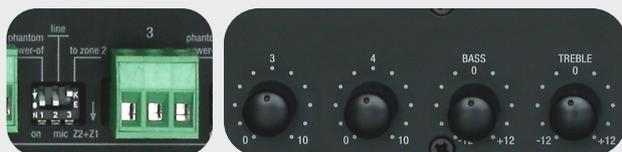
Input 3 is Zone 2 microphone input, which can be assigned to both zones. It also features +24V Phantom Power, and can be switched to support Line level signal. Input level can be adjusted via front panel knob „3“. Tone can be adjusted via combined Input 3 and Input 4 tone controls.
