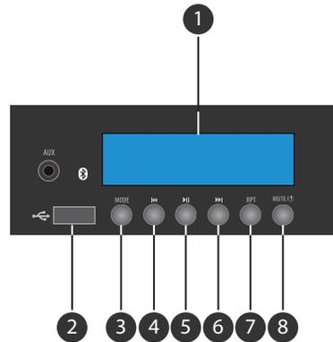
1. LCD screen | 2. USB slot | 3. Mode button | 4. Backward / Set FM frequency and preset | 5. Play-pause / Radio frequency scanning mode
