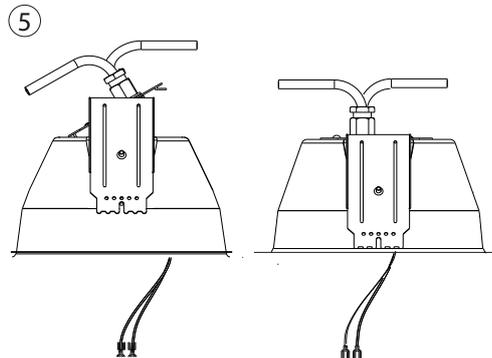
5 Re-fit plate to dome and tighten the wingnut
