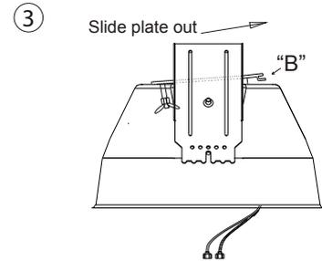
3 Lift the disengaged plates "B" side slightly
