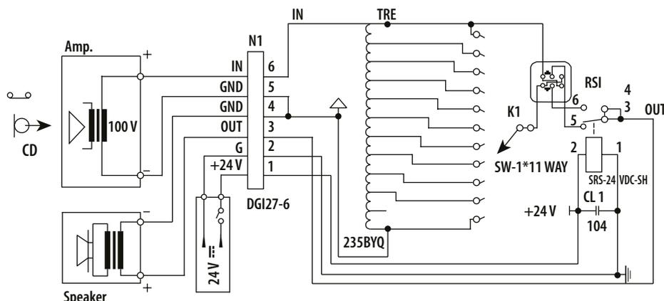
Active mode: Volume control will be fully opened and set to the maximum level until 24V DC is supplied. After DC powering, volume control will come in to operation.
