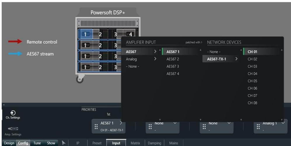
Figure 15 – AES67 input patching window.
