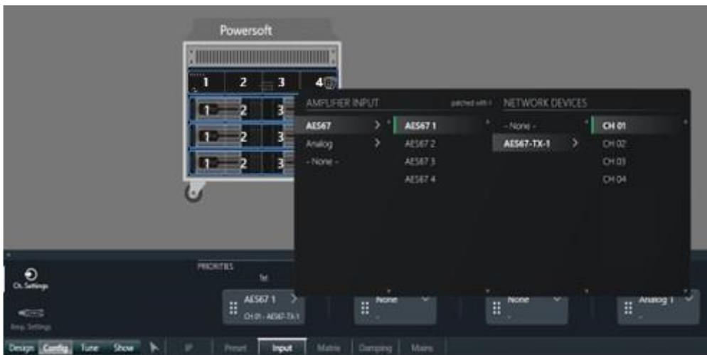
Figure 18 – Patching a Mezzo A+ AES67 Tx to DSP+ Rx.
