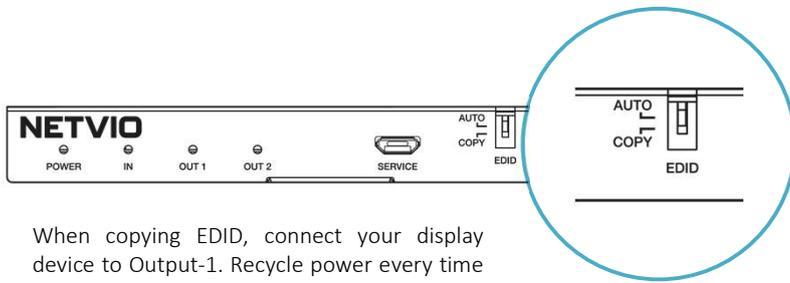
When copying EDID, connect your display device to Output-1. Recycle power every time settings are adjusted.
