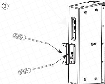
③ Place loudspeaker with attached bracket onto mounting plate. Fix the two security screws on both sides of the bracket to prevent loudspeaker removal from the plate.
