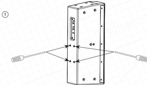
① Unscrew four sockets on the back of loudspeaker. Do not use these removed screws for mounting - proper size screws for attaching bracket are included with RF UB55.
