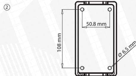
② Attach mounting plate to the surface. Please leave required space from all sides for cables and loudspeaker angle adjustment.
