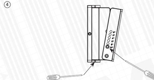
④ Plug audio cables and make final loudspeaker angle adjustments. Place the screws for fixing vertical and horizontal angles and tighten.
