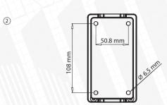
Attach mounting plate to the surface. Please leave required space from all sides for cables and loudspeaker angle adjustment.
