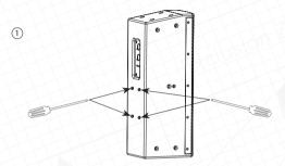
Unscrew four sockets on the back of loudspeaker. Do not use these removed screws for mounting - proper size screws for attaching bracket are included with RF UB55.
