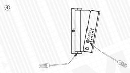
Plug audio cables and make final loudspeaker angle adjustments. Place the screws for fixing vertical and horizontal angles and tighten.
