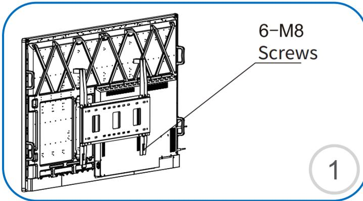
Six M8 screws corresponding to the size of the VESA holes are used to lock the two vertical bar hangers on the VESA mounting holes on the touch screen's back plate.
