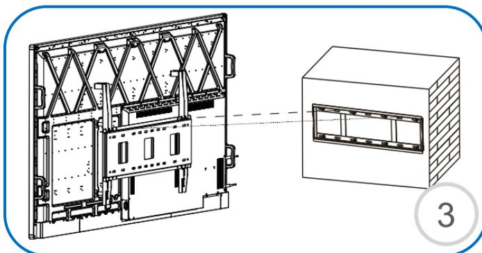
Once the wall bracket is installed and properly secured you may hang the touch screen. You may adjust the left and right position once the screen is in place.
