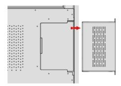
Step 2 Slide the OPS into the OPS port on the rear of the panel until firmly seated.
