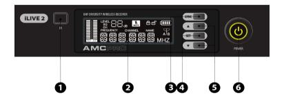
1. IR transmitter | 2. LCD display | 3. SYNC button | 4. SET button | 5. Navigation buttons | 6. Power switch
