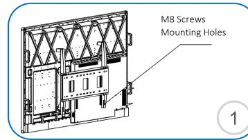
Four M8 screws corresponding to the size of the VESA holes are used to lock the two vertical bar hangers on the VESA mounting holes on the touch screen's back plate.
