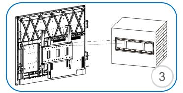
Once the wall bracket is installed and properly secured you may hang the touch screen.
