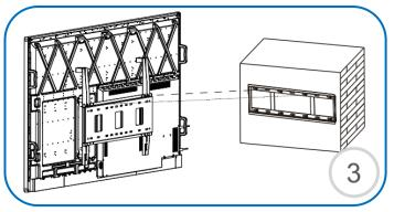
Once the wall bracket is installed and properly secured you may hang the touch screen.
